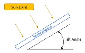
The solar modules must be installed at an angle of at least 10° to the ground. Building regulations must be observed (in Germany maximum 75°).
