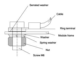
The modules are to be grounded according to the country-specific requirements and laws. If a lightning protection system is already present or intended to be installed on the building, the PV system is to be integrated into the protection concept against direct lightning strike. If a transformerless inverter is used, equipotential bonding may be prescribed in accordance with the inverter manufacturer's specifications. Country-specific laws must be observed.
