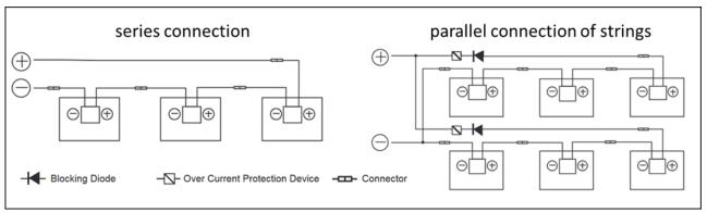
Suitable overcurrent protection measures (e.g. string cut-out) are required for the parallel connection of the solar modules. It must be ensured that the specified capacity regarding the return current IR of the datasheet will not be exceeded. If there are more than two parallel strings, string fuses and string diodes must be used.
