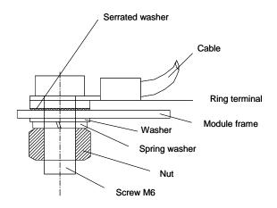
The solar modules are to be grounded according to the country-specific requirements and laws. If a lightning protection system is already present or intended to be installed on the building, the PV system is to be integrated into the protection concept against direct lightning strike. If a transformer less inverter is used, equipotential bonding may be prescribed in accordance with the inverter manufacturer's specifications. Country-specific laws like NEC must be observed.
