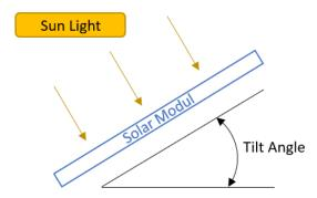
The solar modules must be set up at an angle of at least 10° to the ground. Building regulations must be observed.
